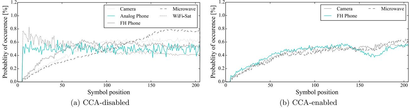
**Figure 8: Symbol error distribution for corrupted 802.15.4 packets (aggregated for packet length 100 byte) interfering with wireless camera, analog phone, FHSS phone, microwave oven, and saturated WiFi.**
