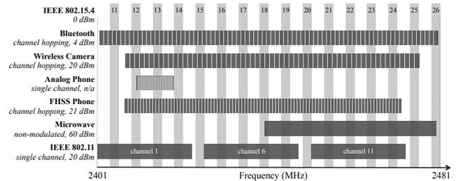
**Figure 1: RF channels of IEEE 802.15.4 and the set of prevalent RF interferers in the 2.4 GHz ISM band studied in this paper.**
