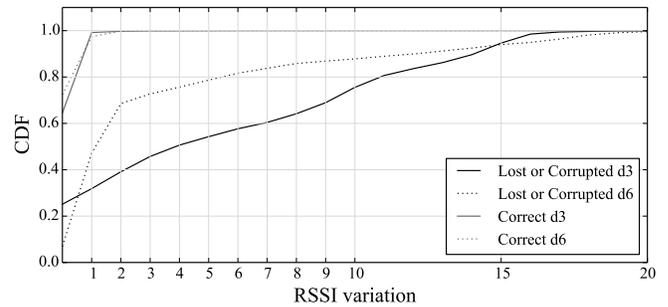
**Figure 7: RSSI analysis based on RSSI samples during packet reception for two distances, 3 (d3) and 6 m (d6), aggregated for all technologies sending at highest transmission power.**
