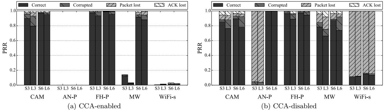
**Figure 4: PRR for CCA-enabled and CCA-disabled traffic types for distances 3 and 6 m. The saturated traffic type follows the same trends as CCA-disabled, hence not shown here. Empty space in CCA-enabled traffic indicates no traffic due to busy medium, i.e., backoff. Bluetooth’s and non-saturated WiFi’s impact on the communication are almost neglectable.**
