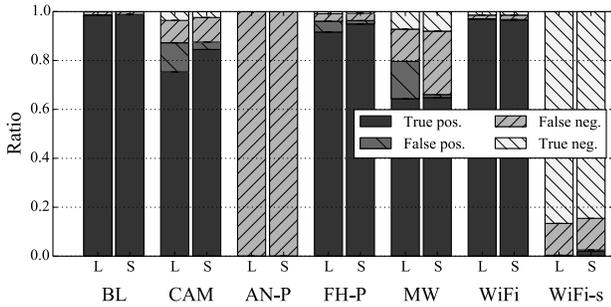
**Figure 9: Ratio of successful or failed back-off decisions with CCA-disabled traffic at distance 6 m with the highest transmission power for 100 byte (L) and 20 byte (S) packets. Distinction between channel free and transmission ok (true positive), channel free but transmission either corrupted or lost (false positive), channel busy but transmission successful (false negative), and channel busy with either corrupted or lost transmission (true negative).**
