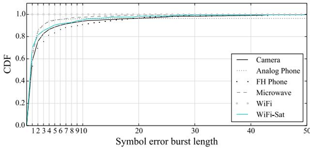
**Figure 6: CDF of symbol error burst lengths considering all corrupted packets.**
