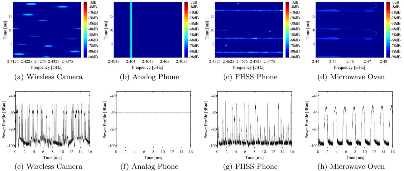
**Figure 3: Characteristics of high-power interferers in the ISM band, in form of spectrograms in first row and power-profiles in the second row.**
