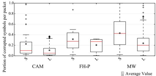
Figure 5: Portion of corrupted symbols in a packet, for the CCA-disabled traffic at distance 6 m for packets with length 100 byte (L) and 20 byte (S).
