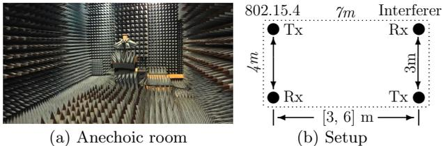
**Figure 2: Experiment setup for the CTI impact study in an anechoic room.**
